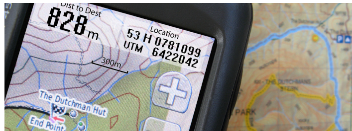
The two 7-digit numbers in the Location field represent a measurement on that map. The Grid Reference here is 810 220 (ie xx810xx and xx220xx)
